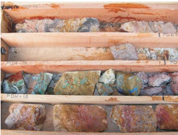
View of PDH 14 and 15 diamond drill core showing skarn with fracture-filling chalcocite and malachite.
