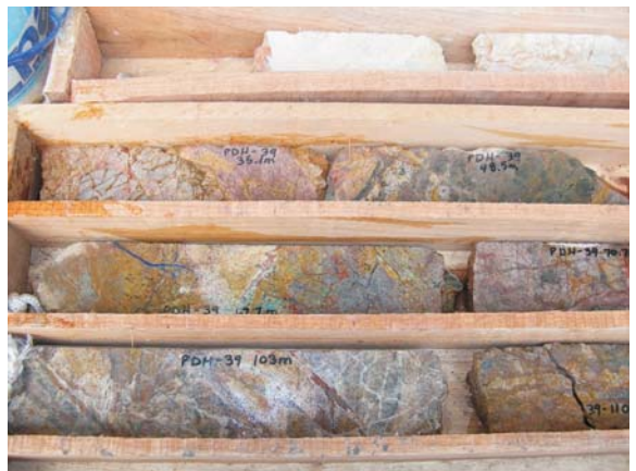
View of PDH 39 diamond drill core showing altered diorite with chalcocite, azurite and malachite.
